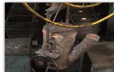
Ladle cover Ceramic wool+MS cover for pouring ladles
